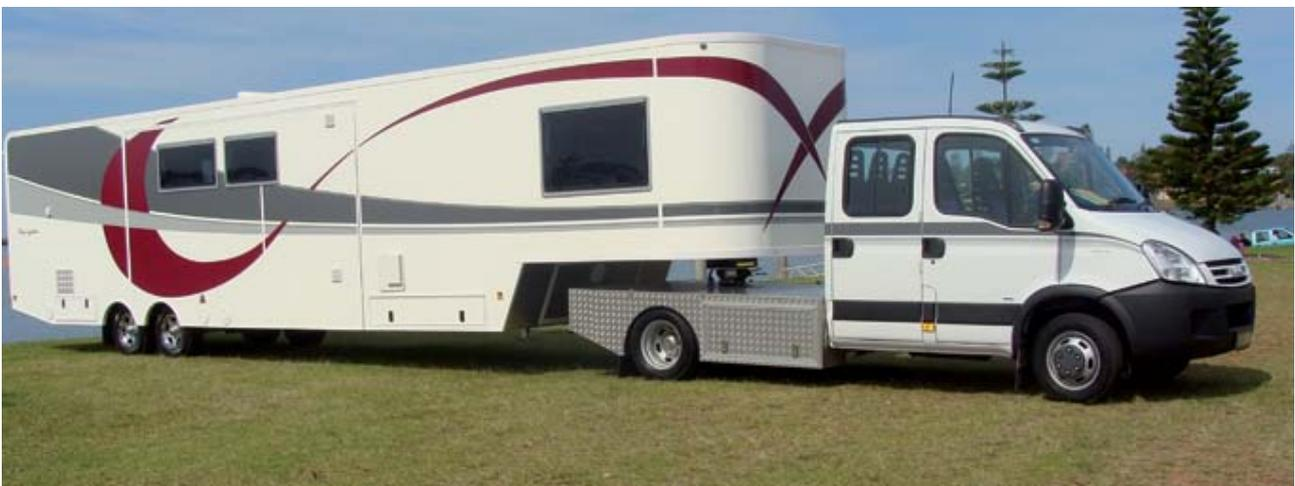
*This 11.3 metre fifth-wheeler built by Glenn Portch is exceptional in weighing only 3200 kg. It has a payload of an extraordinary 1300 kg! Pic: Glenn Portch.*
