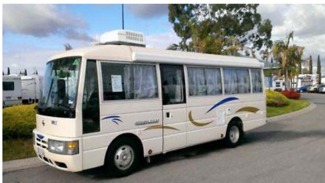
*Roof-mounted air conditioner. Pic: original source unknown.*
