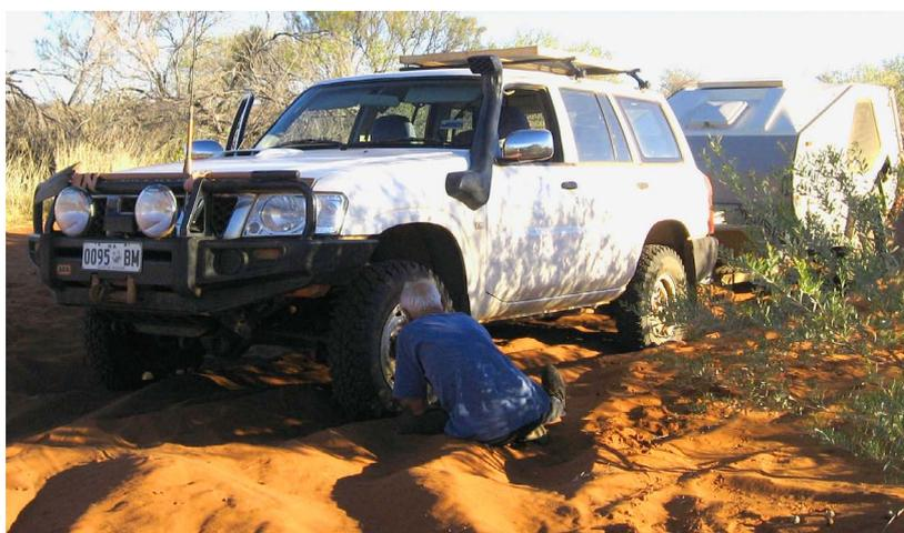
*Reducing tyre pressures on part of the Canning Stock Route to enable progress on the soft track starting here. Pic: Caravan & Motorhome Books.*
